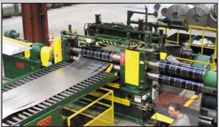
A precision quick-change Turret Head<sup>™</sup> Slitter produces precise width tolerance slit strips with minimum burr throughout the entire range of gauges and mechanical properties. Two (2) quick-change heads allow Magic Steel to conduct an efficient just-in-time production program and respond quickly to customer demands.
