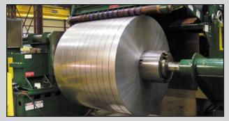
Magic Steel's Slitting Line can produce 20" and 24" ID slit coils. Patented "Speed-Load" Fillers allow Magic Steel to change from 20" to 24" ID (or vice-versa) in one-minute. The Overarm Separator hold-down frame is supported from the inboard and outboard ends to assure the Overarm tooling is square and parallel with the Recoiler drum, assuring straight-walled slit coils. The Overarm features a unique "side-adjust" to allow quick correction of misalignment that might affect coil edge quality.
