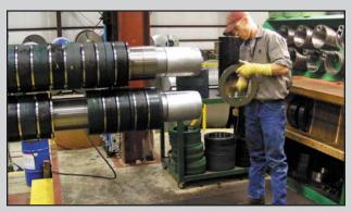
Magic Steel's Turret Head<sup>™</sup> is equipped with two (2) slitter heads supported in massive precision machined solid steel bearing housings. The slitter heads at the "set-up" station are completely
