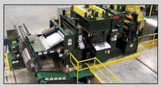
A view of the exit end of Magic Steel's Slitting Line clearly illustrates the compact high-pass line system configuration.
