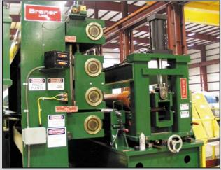
A Non-Marking Belt Tensioner and a Non-Marking "Duplex" Roll Tensioner combine to generate tightly wound straight-walled slit coils. The Belt Tensioner and Duplex Roll Tensioner can be engaged independently or in tandem. The patented Duplex Roll Tensioner is fitted with two (2) sets of tensioning rolls...one set for "wet" strip, and one set for "dry" strip. Switching from wet rolls to dry rolls is accomplished by pushbutton in a matter of minutes.
