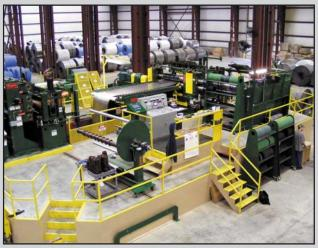
The new Magic Steel Slitter has 750 HP available for processing 60,000# bare, galvanized, and pre-painted coils in widths to 72" at slitting speeds to 1,000 FPM. Coil gauge capacity ranges from 0.009" minimum through 0.135" maximum.
