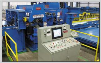
Cascadia's CTL Line features Braner/Loopco's fast and reliable Hi-Speed Hydraulic Shear. Adjustable blade gap allows Cascadia to quickly and easily establish the ideal blade clearance for shearing carbon steel and aluminum alloy throughout the .028" to .250" gauge range. Notable benefits of the Hi-Speed Hydraulic Shear are its exceptional reliability and virtual noise-less shearing cycle.
