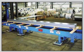
Panel-flat 14-gauge x 14.500" wide x 180" long sheets stacked in straight-sided solid block sheet packs.
