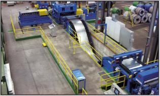
The Longview, WA Cassette Leveler CTL is Cascadia's second Braner/Loopco. Both 72" Hydraulic Cassette Levelers are equipped with 3.000" x 17-roll x 4-Hi and 1.750" x 17-roll x 5-Hi Cassettes that enable Cascadia Metals to produce panel-flat sheets in gauges from 1/4" to .028".
