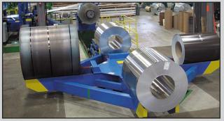
Master coils staged on Cascadia's 4-Station Storage Table show the versatility of the new CTL. Two aluminum alloy coils, a hot rolled, and a thin-gauge pre-painted coil are in the queue awaiting the tail-out of a galvanized coil being processed.
