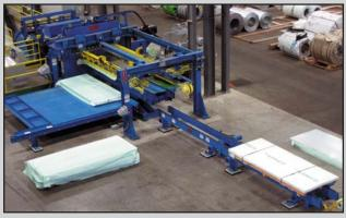
A finished sheet pack awaits removal while a new pack is being generated in the Stacker. A fresh skid placed on the Injector Table awaits injection into the Stacker.
