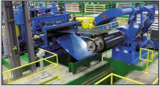
60,000# x 72" wide master coils are transferred via Coil Car from the Storage Table to the Uncoiler. A laser aligns the coil on the Uncoiler while a fiber optic Edge Guide maintains coil alignment while running. A Crop Shear prepares the coil head end for threading and "splits" coils that are partial runs.
