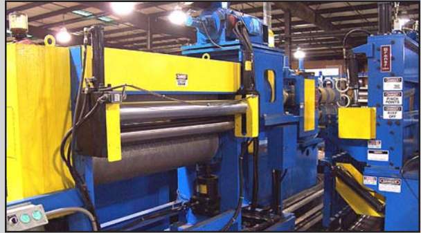
Embosser is set-up to be injected in and out of the line
