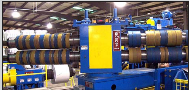
Turret Head™ Slitter exchanges slitter heads in less than 2-minutes
