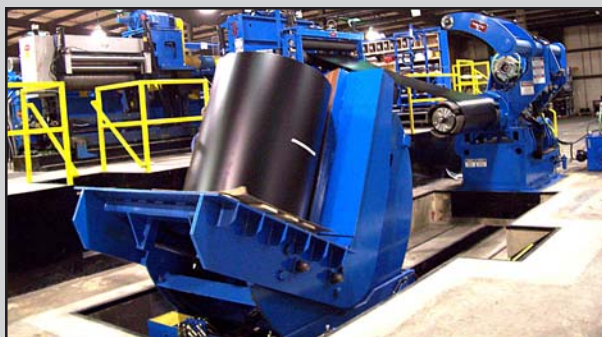
Entry Coil Car-Tipper upends and loads coils onto the Uncoiler
