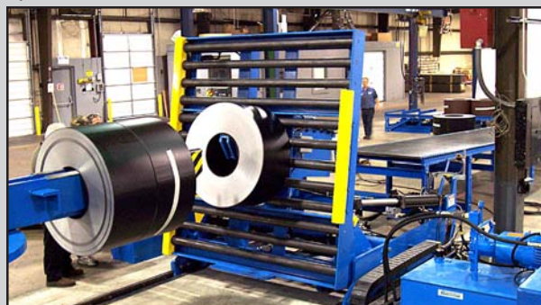
Operatorless Programmable Downender retrieves slit coils from the 4-Arm and sends the coils to a Strapping Machine and Coil Stacker.
