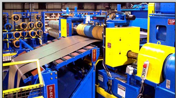
Surface inspection is accomplished as the strip leaves the Slitter
