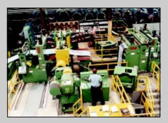
The slitting line is a high pass line "Generation V" coil slitting system designed for fast coil threading and quick job changeovers. The high pass line design takes full advantage of the natural coil set for extremely fast coil threading, and eliminates coil breaks induced by reverse bending the strip as is common on low pass line slitters.
