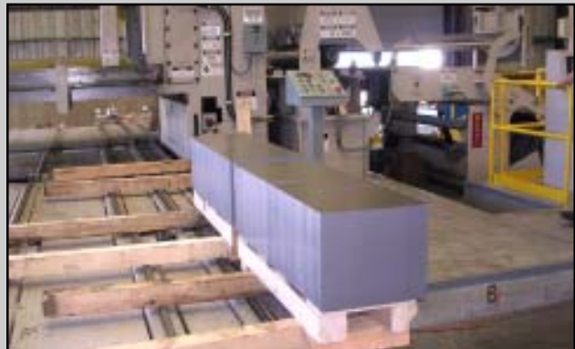
Programmable Stacker Produces Solid-Block Multi-Blank Stacks
